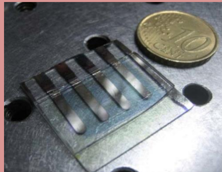
Four ErQ-based IR OLEDs on a single glass substrate
